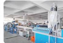
9 Automatic pneumatic tube manufacturing lines
