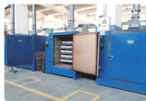
Spray paint oven
