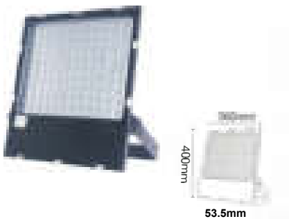
MODE:HTD-EL5028055 POWER:120W SIZE:400*360*53.5mm IN PUT VOITAGE:AC85-265V / AC24V /DC24V MATERIAL:aluminum Toughened glass PROTECTION CLASS:IP65 LIGHT EFFICIENCY:80lm/W Ra=80 ANGLE:10°15°24°30°45°60°90°
