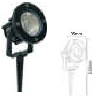
MODE: HTD-EL5023056 POWER: 7W COB SIZE: D95*H310mm INPUT VOITAGE: AC85-265V/AC12/24V/DC12/24V MATERIAL: aluminum Toughened glass PROTECTION CLASS: IP65 LIGHT EFFICIENCY: 80lm/W Ra=90 ANGLE: 24°
