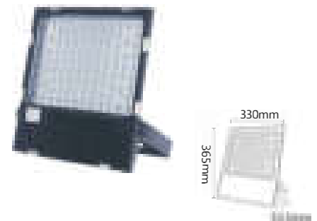
MODE:HTD-EL5028054 POWER:100W SIZE:365*330*53.5mm INPUT VOITAGE:AC85-265V/AC24V/DC24V MATERIAL:aluminum Toughened glass PROTECTION CLASS:IP65 LIGHT EFFICIENCY:80lm/W Ra=80 ANGLE:10°15°24°30°45°60°90°
