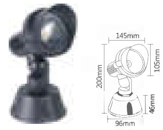
MODE:HTD-EL5023071-A POWER:5W/7W COB SIZE:D105*H200mm INPUT VOITAGE:AC85-265V/AC12/24V/DC12/24V MATERIAL:aluminum Toughened glass PROTECTION CLASS:IP65 LIGHT EFFICIENCY:80lm/W Ra=90 ANGLE:24°
