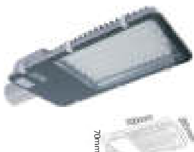
MODLE:HTD-EL5027061 POWER:150W SIZE:700*285*70mm INPUT VOITAGE:AC85-265V MATERIAL:aluminum Toughened glass plastic PROTECTION CLASS:IP65 LIGHT EFFICIENCY:100lm/W Ra=80
