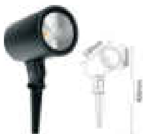
MODE:HTD-EL5023281 POWER:12W COB SIZE:D90*H400mm INPUT VOITAGE:AC85-265V/AC12/24V/DC12/24V MATERIAL:aluminum Toughened glass PROTECTION CLASS:IP65 LIGHT EFFICIENCY:80lm/W Ra=90 ANGLE:24°
