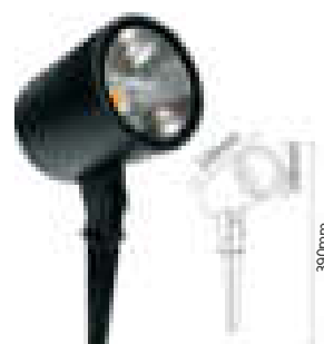
MODE:HTD-EL5023283 POWER:18W COB SIZE:D108*H390mm INPUT VOITAGE:AC85-265V/AC12/24V/DC12/24V MATERIAL:aluminum Toughened glass PROTECTION CLASS:IP65 LIGHT EFFICIENCY:80lm/W Ra=90 ANGLE:24°
