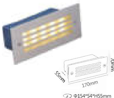
MODE:HTD-EL5021050 POWER:5W SIZE:170*70*55mm INPUT VOITAGE:AC85-265V/AC12/24V/DC12/24V MATERIAL:201SS aluminum Toughened glass plastic PROTECTION CLASS:IP65 LIGHT EFFICIENCY:35lm/W Ra=80
