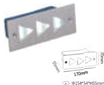
MODE:HTD-EL5021052 POWER:5W SIZE:170*70*55mm INPUT VOITAGE:AC85-265V / AC12/24V /DC12/24V MATERIAL:201SS aluminum Toughened glass plastic PROTECTION CLASS:IP65 LIGHT EFFICIENCY:35lm/W Ra=80
