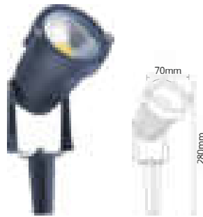
MODE: HTD-EL5023003 POWER: 5W COB SIZE: D70*H280mm INPUT VOITAGE: AC85-265V/AC12/24V/DC12/24V MATERIAL: aluminum Toughened glass PROTECTION CLASS: IP65 LIGHT EFFICIENCY: 80lm/W Ra=90 ANGLE: 36°
