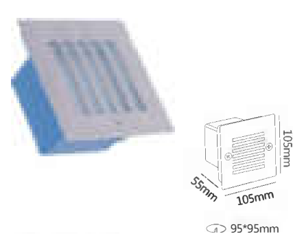
MODE:HTD-EL5021055 POWER:5W SIZE:105*105*55mm INPUT VOITAGE:AC85-265V / AC12/24V /DC12/24V MATERIAL:201SS aluminum Toughened glass plastic PROTECTION CLASS:IP65 LIGHT EFFICIENCY:35lm/W Ra=80
