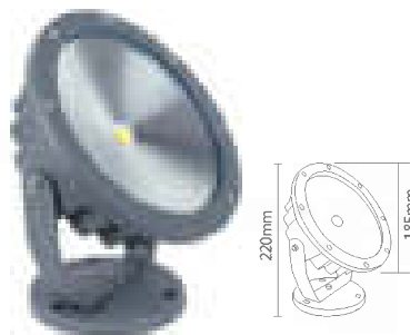
MODE: HTD-EL5023007 POWER: 20W COB SIZE: D185*H200mm INPUT VOITAGE: AC85-265V/AC12/24V/DC12/24V MATERIAL: aluminum Toughened glass PROTECTION CLASS: IP65 LIGHT EFFICIENCY: 80lm/W Ra=90 ANGLE: 60°
