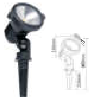
MODE:HTD-EL5023072-B POWER:5W/7W COB SIZE:D105*H300mm INPUT VOITAGE:AC85-265V/AC12/24V/DC12/24V MATERIAL:aluminum Toughened glass PROTECTION CLASS:IP65 LIGHT EFFICIENCY:80lm/W Ra=90 ANGLE:24°
