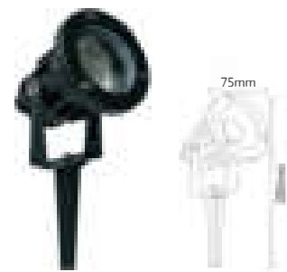
MODE: HTD-EL5023066 POWER: 5W COB SIZE: D75*H280mm INPUT VOITAGE: AC85-265V/AC12/24V/DC12/24V MATERIAL: aluminum Toughened glass PROTECTION CLASS: IP65 LIGHT EFFICIENCY: 80lm/W Ra=90 ANGLE: 24°
