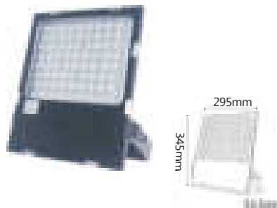
MODE:HTD-EL5028053 POWER:50W SIZE:345*295*53.5mm IN PUT VOITAGE:AC85-265V / AC24V /DC24V MATERIAL:aluminum Toughened glass PROTECTION CLASS:IP65 UGHT EFFICIENCY:80lm/W Ra=80 ANGLE:10°15°24°30°45°60°90°
