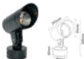
MODE:HTD-EL5023284-A POWER:7W COB SIZE:D65*H200mm INPUT VOITAGE:AC85-265V/AC12/24V/DC12/24V MATERIAL:aluminum Toughened glass PROTECTION CLASS:IP65 LIGHT EFFICIENCY:80lm/W Ra=90 ANGLE:24°
