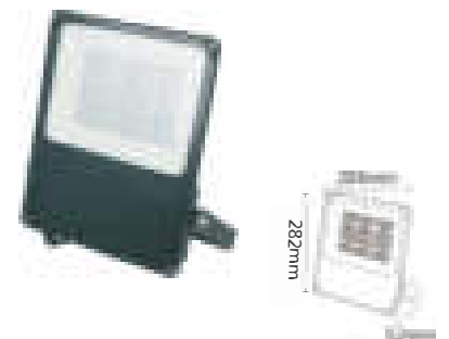
MODE:HTD-EL5028059 POWER:50W SIZE:282*204*52mm INPUT VOITAGE:AC85-265V MATERIAL:aluminum Toughened glass PROTECTION CLASS:IP65 LIGHT EFFICIENCY:100lm/W Ra=80 ANGLE: 30° 60° 90° 120°
