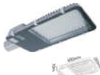
MODLE:HTD-EL5027060 POWER:120W SIZE:600*265*70mm INPUT VOITAGE:AC85-265V MATERIAL:aluminum Toughened glass plastic PROTECTION CLASS:IP65 UGHT EFFICIENCY:100lm/W Ra=80
