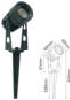
MODE:HTD-EL5023001 POWER:3W/5W COB SIZE:D40*H250mm INPUT VOITAGE:AC85-265V/AC12/24V/DC12/24V MATERIAL:aluminum plastic PROTECTION CLASS:IP65 LIGHT EFFICIENCY:80lm/W Ra=90 ANGLE:24°
