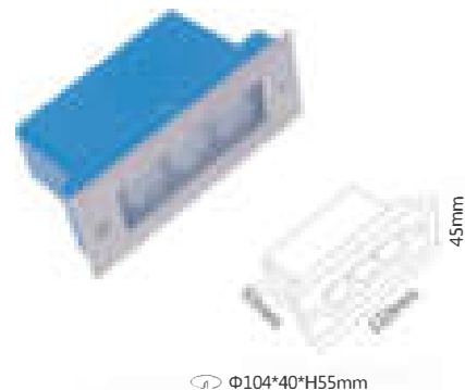
MODE:HTD-EL5021090 POWER:3W SIZE:110*45*55mm INPUT VOITAGE:AC85-265V / AC12/24V /DC12/24V MATERIAL:201SS aluminum Toughened glass plastic PROTECTION CLASS:IP65 LIGHT EFFICIENCY:80lm/W Ra=80 ANGLE:5°10°15°24°30°45°60°90°
