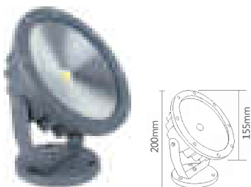
MODE: HTD-EL5023006 POWER: 15W COB SIZE: D155*H200mm INPUT VOITAGE: AC85-265V/AC12/24V/DC12/24V MATERIAL: aluminum Toughened glass PROTECTION CLASS: IP65 LIGHT EFFICIENCY: 80lm/W Ra=90 ANGLE: 60°
