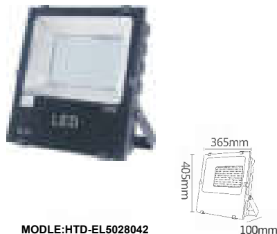
MODE:HTD-EL5028042 POWER:240W SIZE:405*365*100mm INPUT VOITAGE:AC85-265V MATERIAL:aluminum Toughened glass PROTECTION CLASS:IP65 UGHT EFFICIENCY:100lm/W Ra=80 ANGLE:120°
