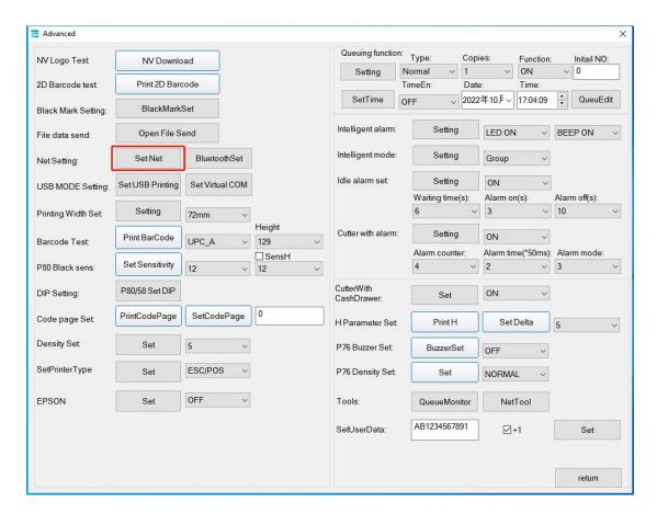
(3) Set the IP of the printer WiFi(note that the IP needs to be set in the same gateway as the home network), and the printer is connected to the home nerwork
