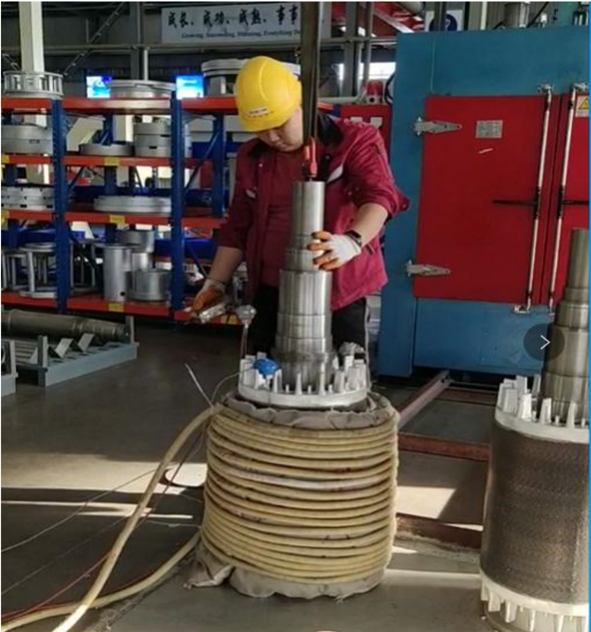
MYD-80KW for motor shell heating for thermal assembly temperature 200°C
