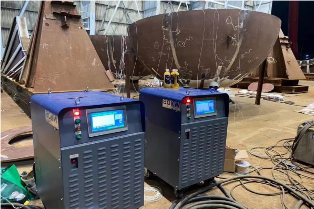
MYD-80KW PWHT Equipment for Pressure Vessel PWHT(Blanket coils)
