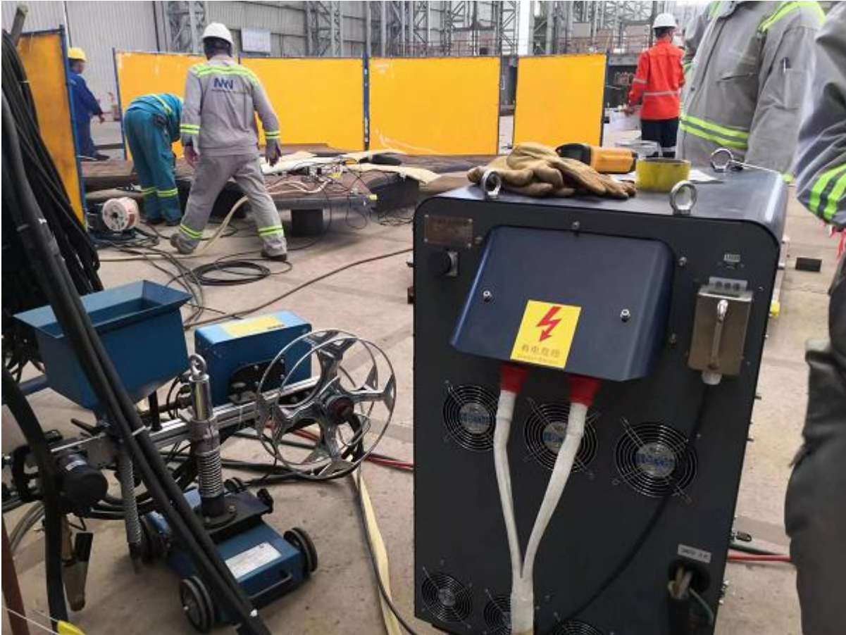
MYD-80KW PWHT700-Offshore Platforms Steel Structure Thickness 80mm
