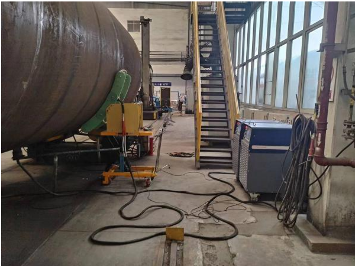
MYD PWHT700 Equipment +C shape Coil for Pressure vessel preheat and heat treatment
