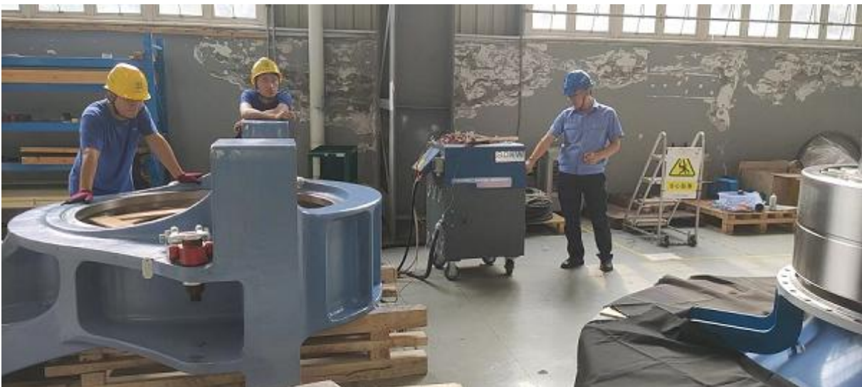
MYD-80KW for motor shell heating for thermal assembly temperature 200°C
