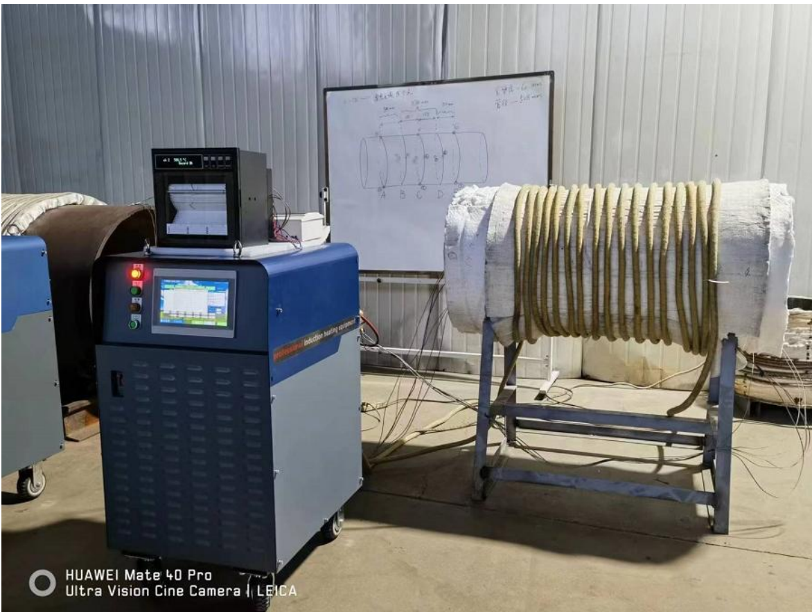
Pipeline PWHT with Soft Cable Coil with 12 Channels Heating Curve
