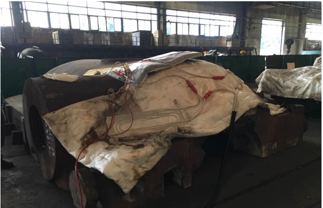
Preheating and post weld heat treatment for repair welding of thick walled castings
