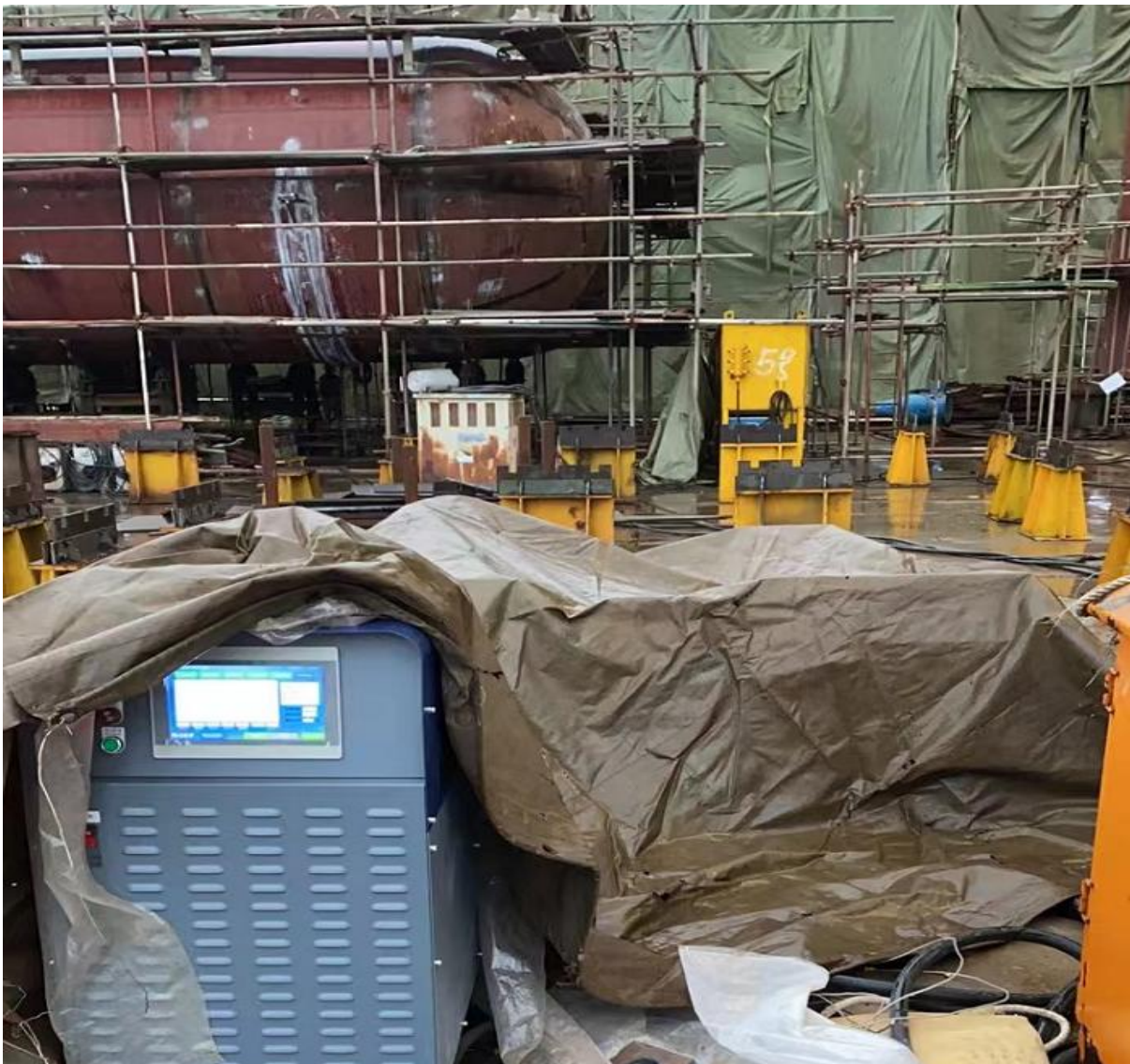
MYD-80KW PWHT Equipment for Pressure Vessel PWHT(Blanket coils)
