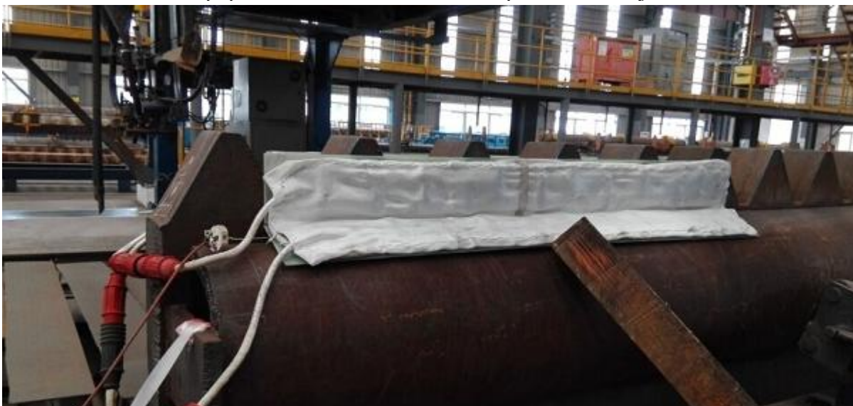
MYD-40KW PWHT equipment for steel structure weld preheat- Fillet joint
