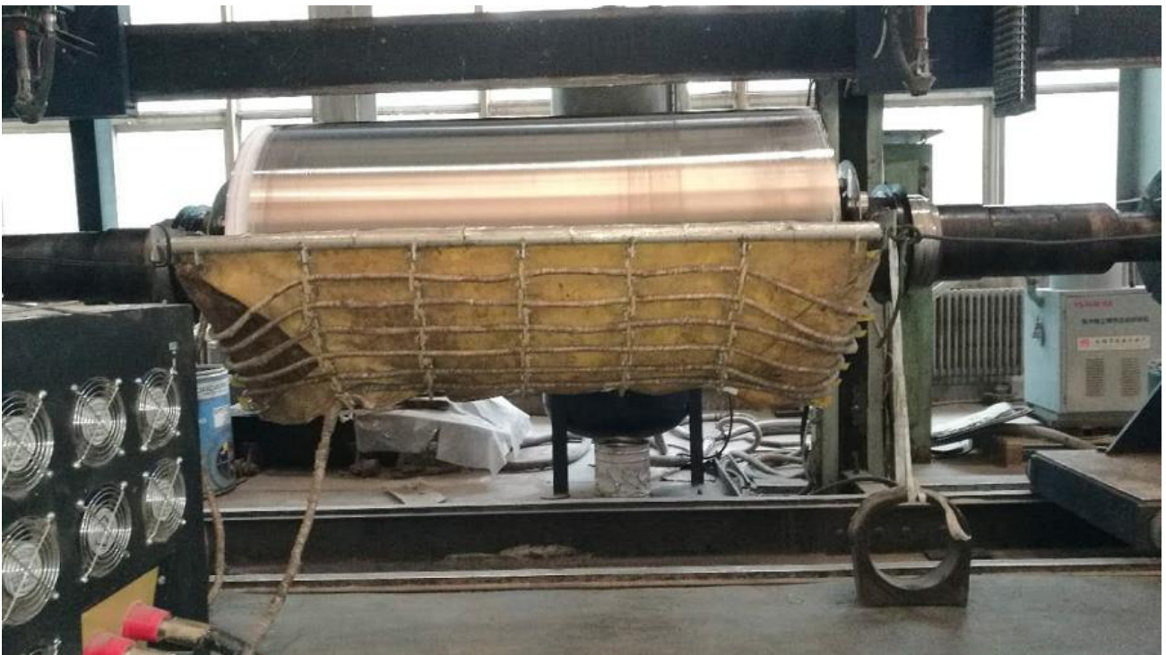
Preheating and post weld heat treatment for roller surfacing
