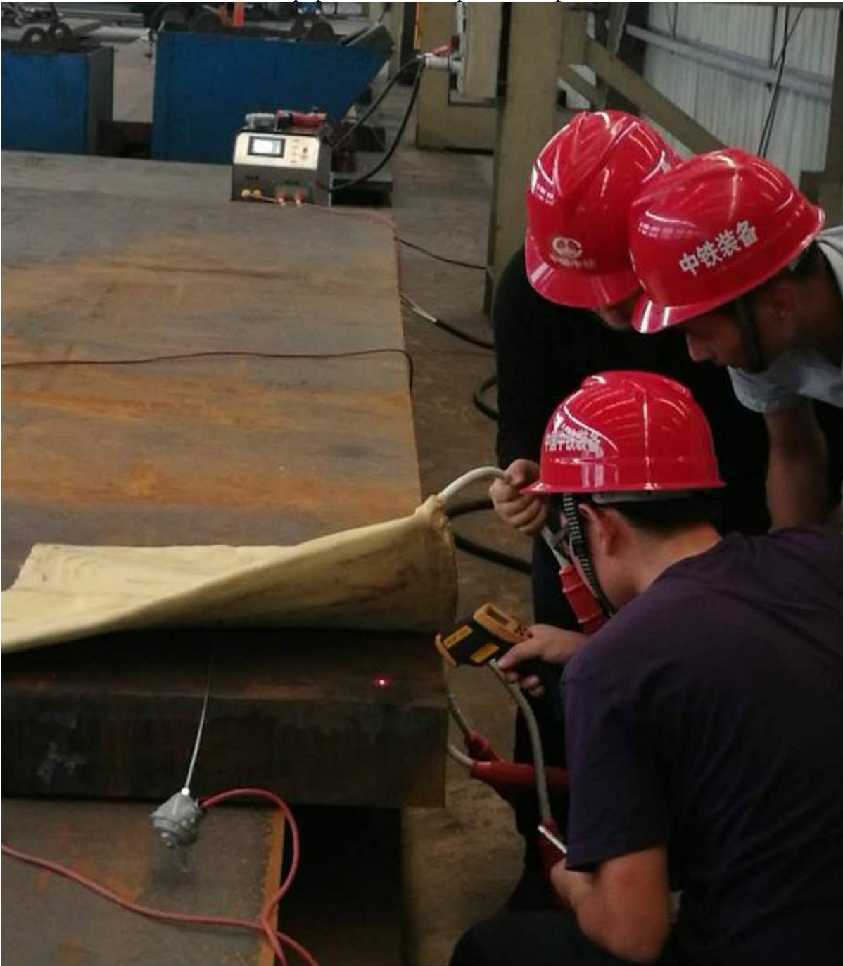
MYD-40KW PWHT equipment for steel structure weld preheat- Fillet joint
