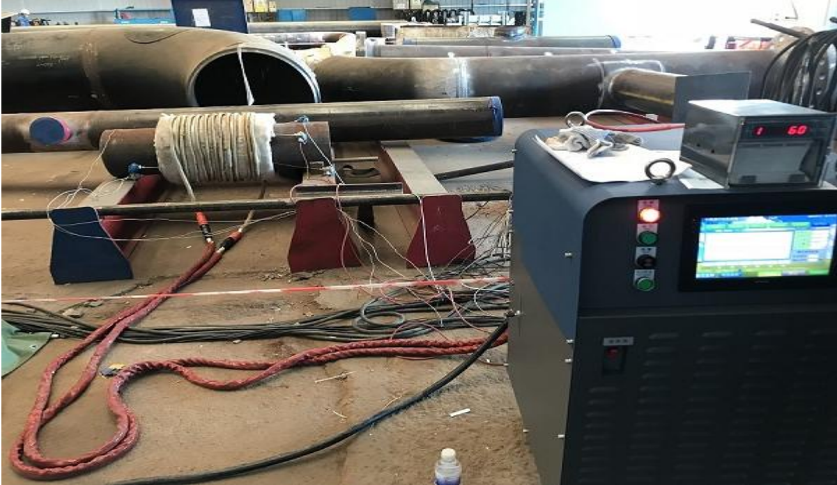
Pipeline PWHT with Soft Cable Coil with 12 Channels Heating Curve
