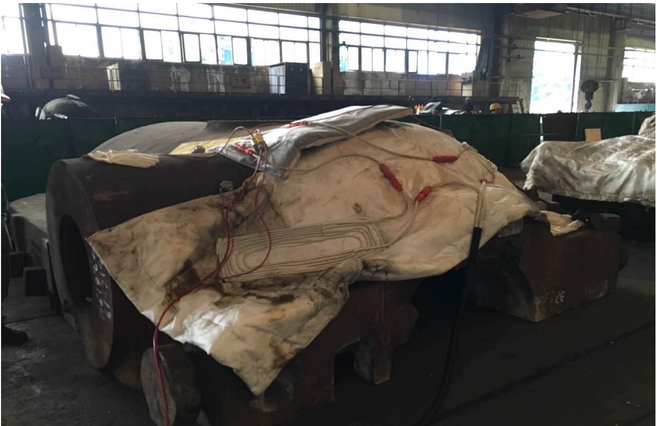
Preheating and post weld heat treatment for repair welding of thick walled castings
