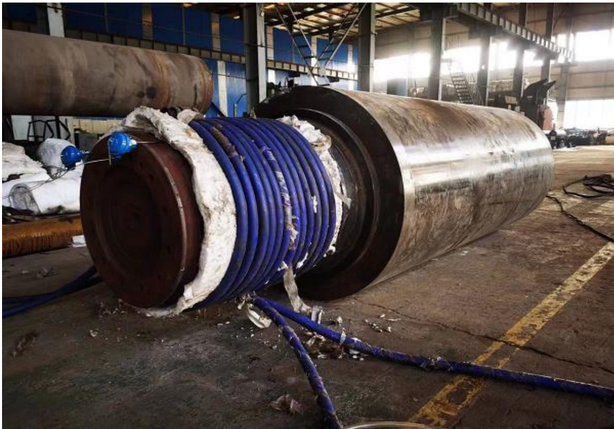
MYD-120KW PWHT Equipment with 30m Soft Cable Coil(water cooled)
