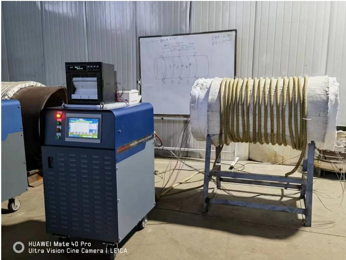
MYD-120KW PWHT Equipment with 30m Soft Cable Coil(water cooled)
