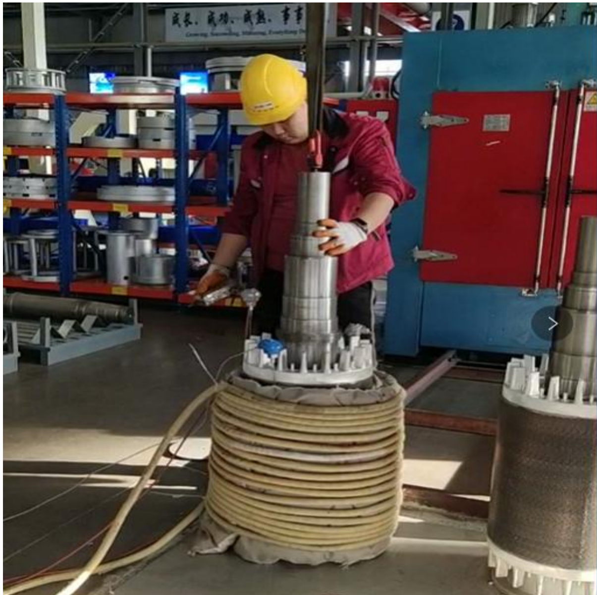
MYD-80KW for motor shell heating for thermal assembly temperature 200°C
