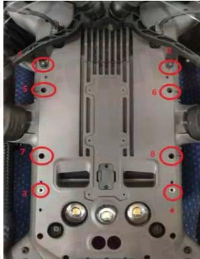
As shown above, with the mounting plate on the left, fix the 1.2.3.4 hole positions to the 5.6.7.8 holes under the M300 large plate on the right.
