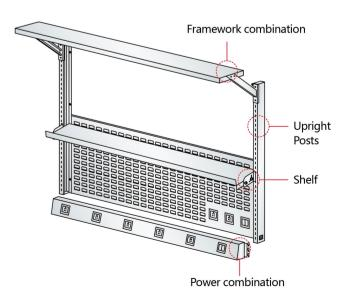
Connection holes and connection pins come as standard factory configuration.
