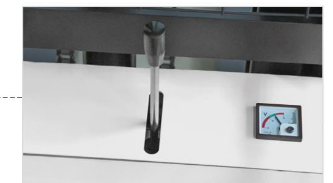
Use handle to control fork height electrically
