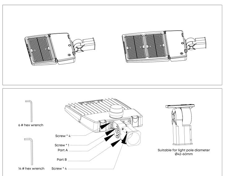
If the lamp is installed through a lamp post, please loosen the screws that fix the two brackets first, then adjust the brackets to their positions. After adjustment, tighten the screws with a 14# hexagonal wrench to fix the brackets, as shown in the figure below.
