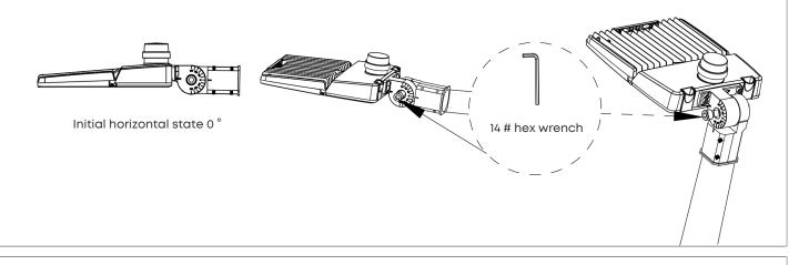
5. Rotate the lamp to the appropriate angle according to actual needs, and then tighten the fixing screws on the bracket
