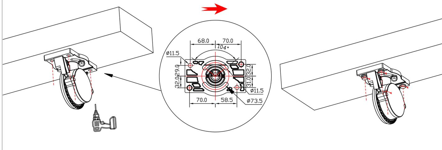
3. Thread the cable out of the bracket.
