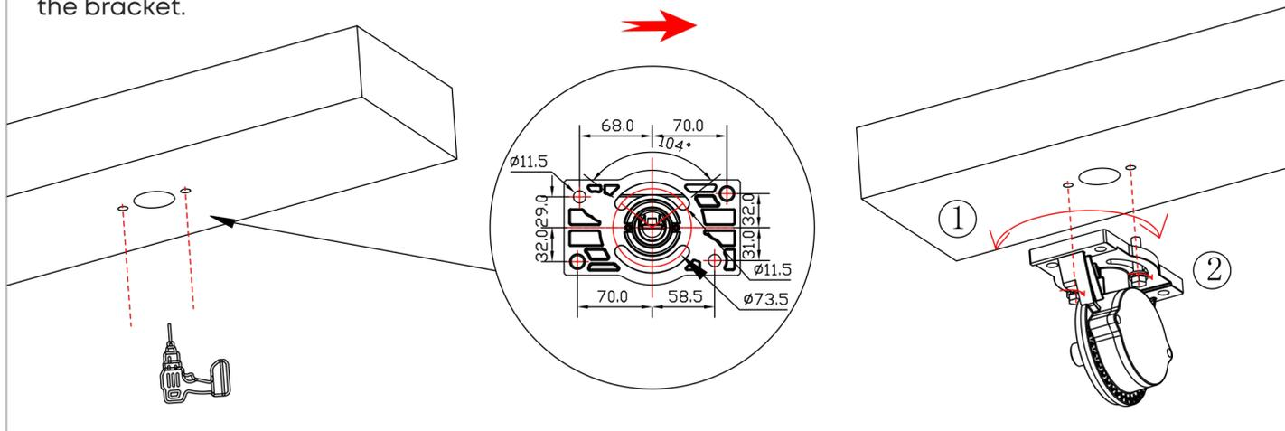
2. Drill holes in the lamp post according to the bracket's hole position and tighten the screws.
