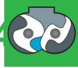
The female rotor exposes the outlet port and the compressed air is delivered to the system.
