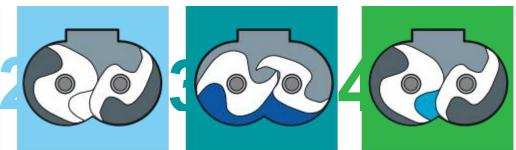
Air is trapped between the teeth of the male and female rotors.
