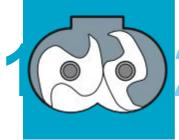
Atmospheric air is drawn through the inlet port into the compressor chamber as a result of the rotational action of the tooth rotors.
