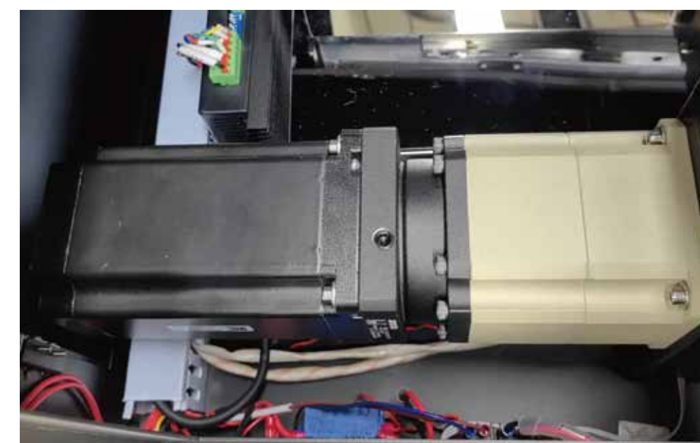
High-power deceleration stepping motor for stable operation
