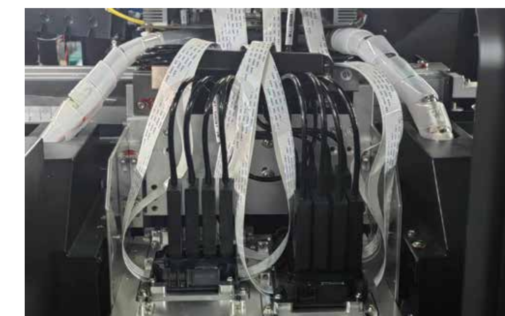
Special UV long damper, more stable ink supply
