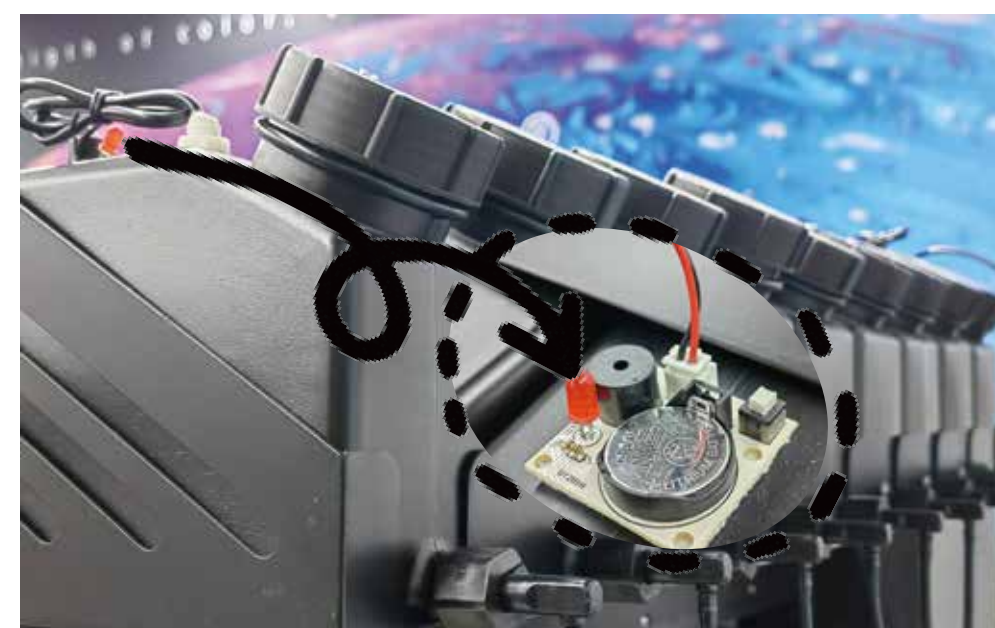
1.5L large capacity ink tank ink tank shortage alarm device
