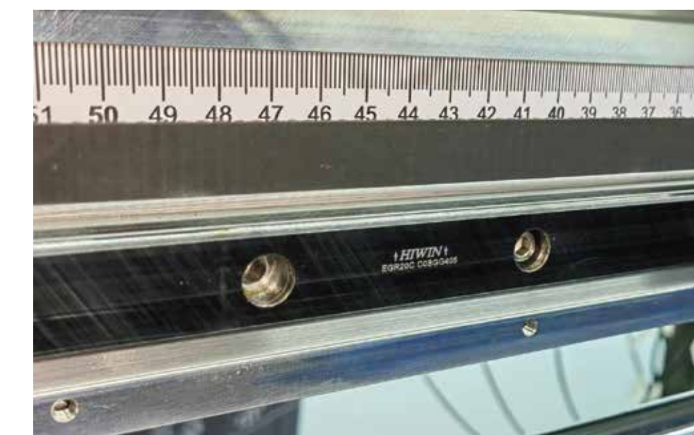
HIWIN high-precision linear guide, print more smoothly
