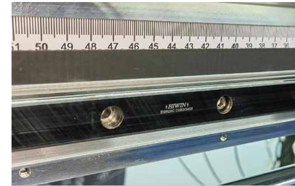
HIWIN high-precision linear guide, print more smoothly
