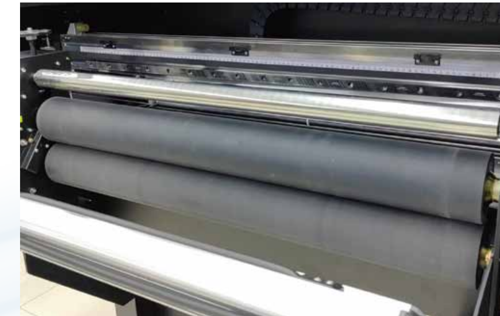
Thickened laminating rubber roller
