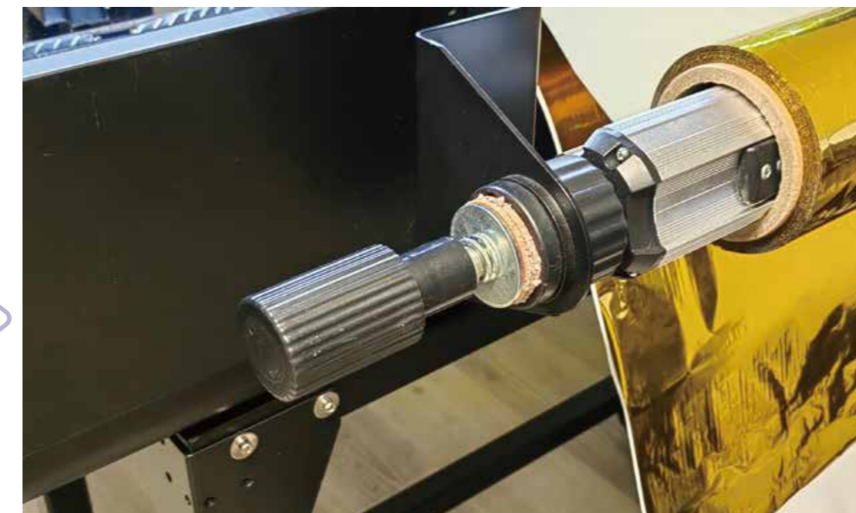
Enlarged front tensioning handle of film rod
