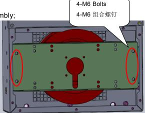
10.3 How to replace the PCB- Printed Circuit Board 如何更换线路板
