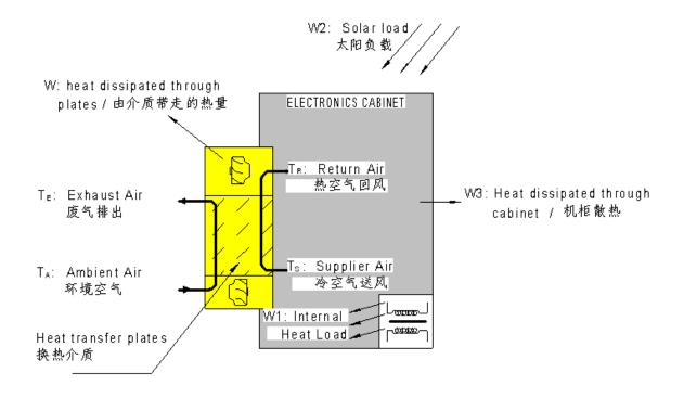
Heat exchanger is mostly used for enclosed area cooling, HEX is designed especially for mounting in a cabinet. The unit uses ambient air for temperature regulation so it must have access to ambient. The internal temperature of the enclosure is cooled via effective utilization of the ambient air. An air/air counter-current plate heat exchanger is used to transfer the heat. Two centrifugal fans, one for the internal circuit and one for the external circuit provide ventilation.
