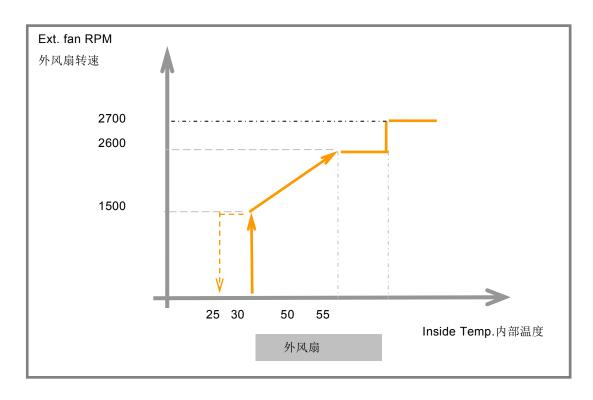
The fan speeds are monitored via the tacho output from the fans. This tacho signal is also used to generate a fan failure signal if deviation is more than -20%. The PWM carrier frequency is 1KHz. 风扇转速是通过风扇的调速装置来调节的,当转速偏差-20%以上时,这个调速装置会产生一个风扇失效信号。调速频率为1K赫兹。
