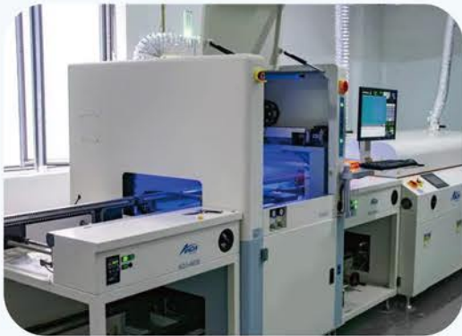
Conformal Coating Machine
