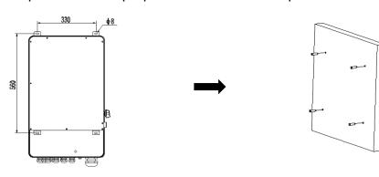
**Step 2**: Lift the inverter and align the hole of the inverter with the expansion bolt, Fix the inverter on the wall.
