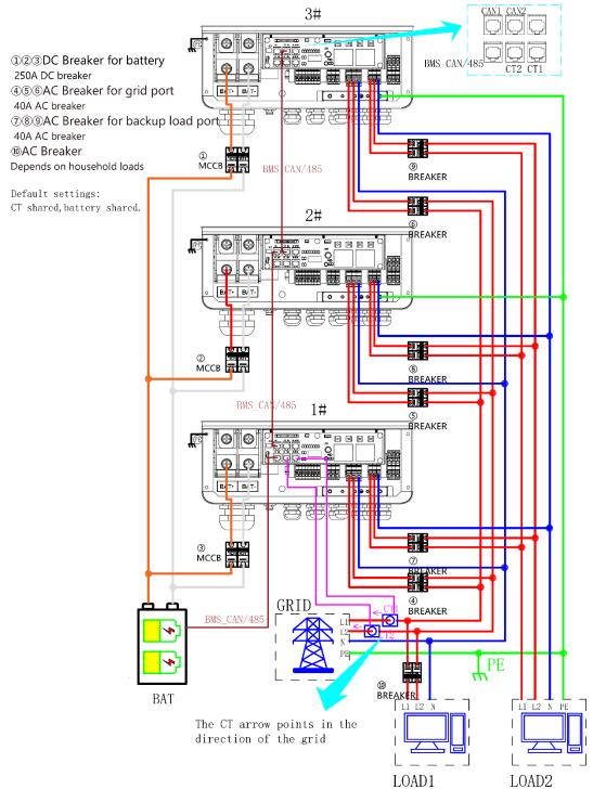
**Note:** Supports up to 3 machines connected in parallel.
