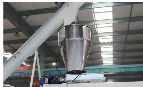
Dosing feeder unit
