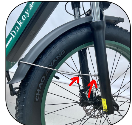
Installing the fenders on the shocks (Shocks come with screws and spacers)
