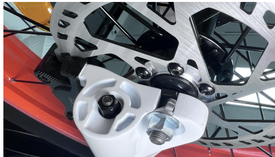
A16. Fork dropouts hold the tips of the hub axle
