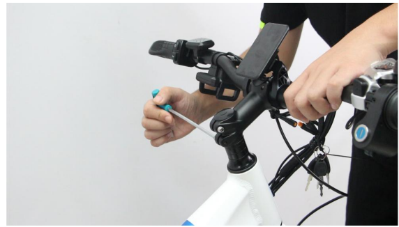
A10. Turn the 2 bolts on both sides to tighten the stem
