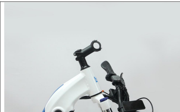
A05. The correct direction the stem should be facing
