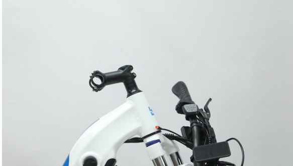
A03. The arch of the fork should be facing forward
