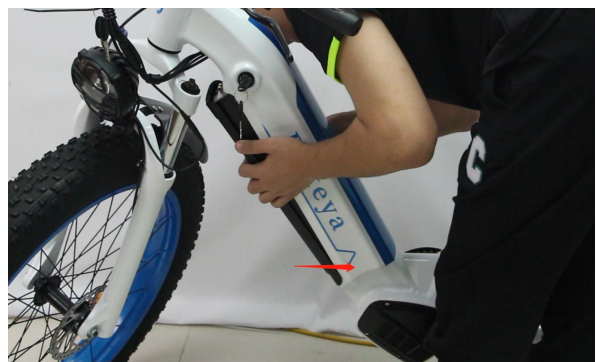
A37. Push the battery to install it tightly
