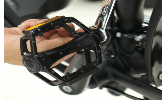
A34. Turn spanner counter-clockwise to fix the pedal L on the left side
