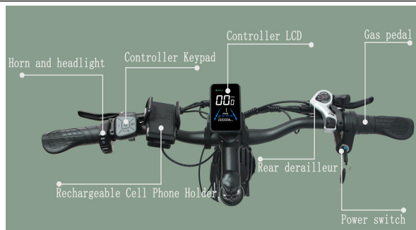
A40. Turn the key on the handlebar first and then press button Power ON/OFF for 3 seconds on the display to turn on power.
