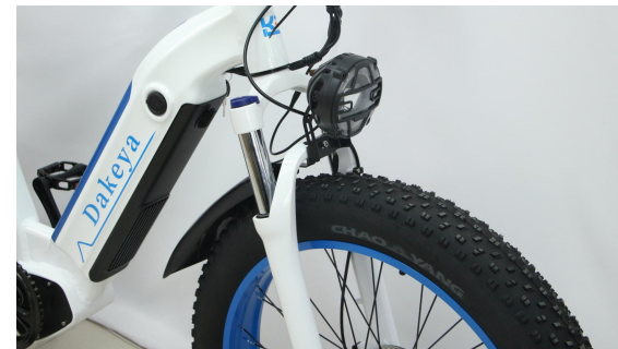
A25. The headlight and fender are fixed on the fork arch
