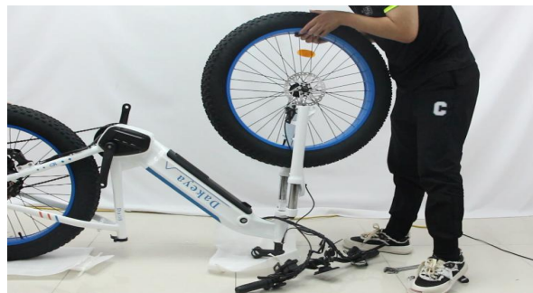
A15. Put the front wheel on the fork
