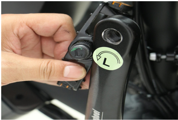
A34. Turn spanner counter-clockwise to fix the pedal L on the left side
