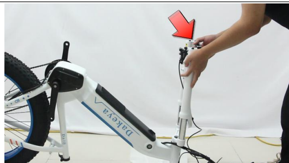
A13. Remove the fork spacer. (it protects the fork from crushing and deformation during shipping, it is not a part of the bike )
