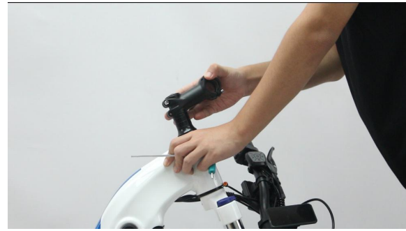
A04. Turn the stem forward ( do not turn the whole fork )
