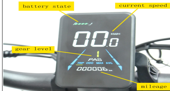
A41. LCD Display: battery status, real-time speed, speed grade, Mileage traveled
