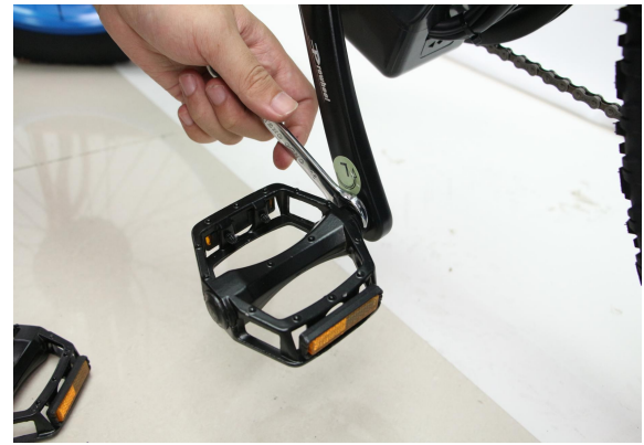
A34. Turn spanner counter-clockwise to fix the pedal L on the left side
