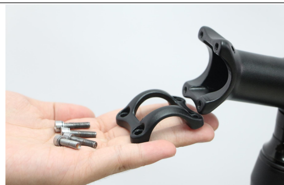
A06. Remove the 4 bolts
