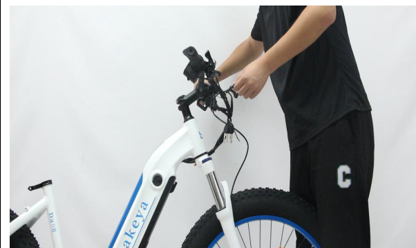
A07. The correct orientation of the handlebar
