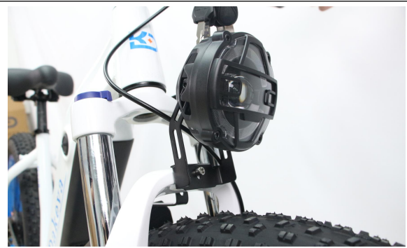
A23. Use the bolt to join the headlight, fork arch and fender
