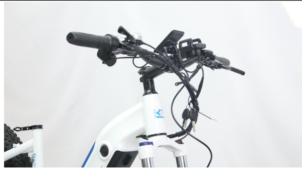
A09. Tighten the 4 bolts to fix handlebar
