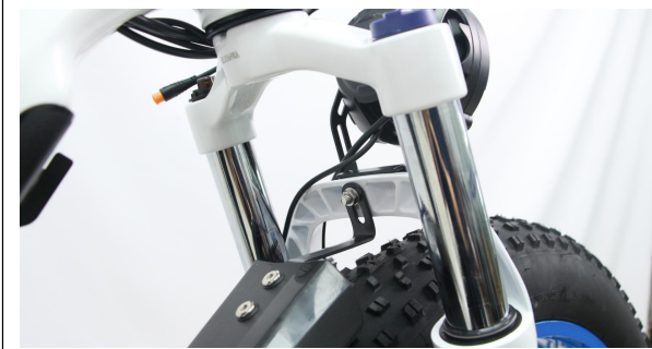
A24. details of the bolt that join headlight and fender together
