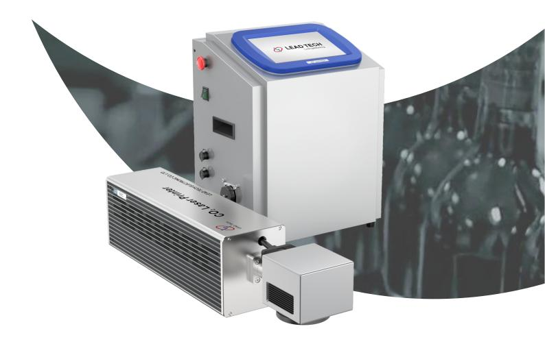
LEAD TECH New Compact CO2 laser marking machine is designed for providing high quality codes for large-scale substrates and is easy to integrate for most of applications. It is an ideal solution for marking on PET bottles, plastics, PP/PE films, boxes, cartons and other primary coding applications to produce high quality visible codes at fast speed with nearly zero maintenance and no consumables required.
