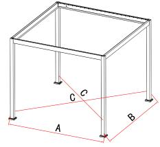
Measure the diagonal and line distance between two posts, ensure size correct, then fasten other two posts.
