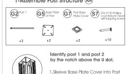
2.Use ST4.2\*30 Phillips countersunk head self-tapping screw fasten base
