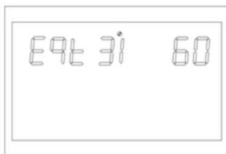
Figure 1-48 Equalization charging time setting(page)
