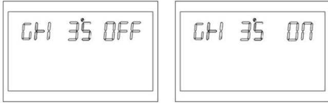
Figure 1-52 The grid-connected inverter function setting page
