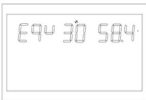
Figure 1-47 Equalization voltage point setting page
