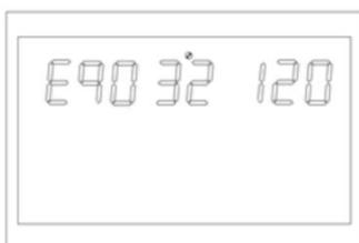
Figure 1-49 Equalization Delay Time Settings Page
