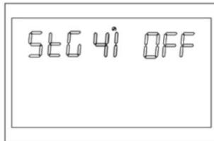
Figure 1-58 Low SOC to mains function setting page
