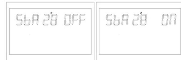
Figure 1-45 Missing battery alarm page
