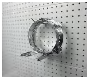
Cap rings 16 sets snap into cap station for embroidery preparation
