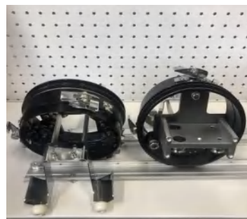
270° cap driver 8 sets snaps into bracket holder for the machine hoops
