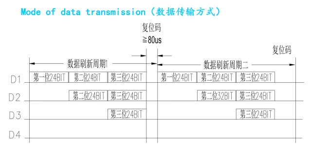
Note: D1 is the data sent by the MCU, and D2, D3, and D4 are the data that the cascade circuit automatically reshapes and forwards.
