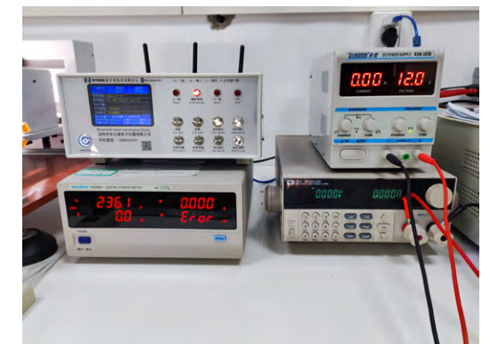
Power test, grounding safety test, dielectric strength test
