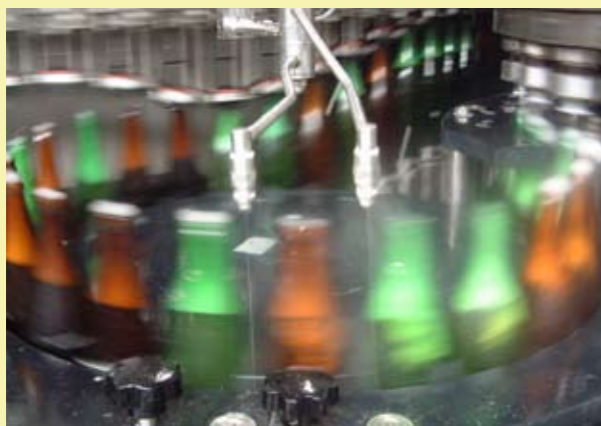
高压激泡减少 瓶颈空气含量 Drop air content in the bottle neck with high pressure foam
