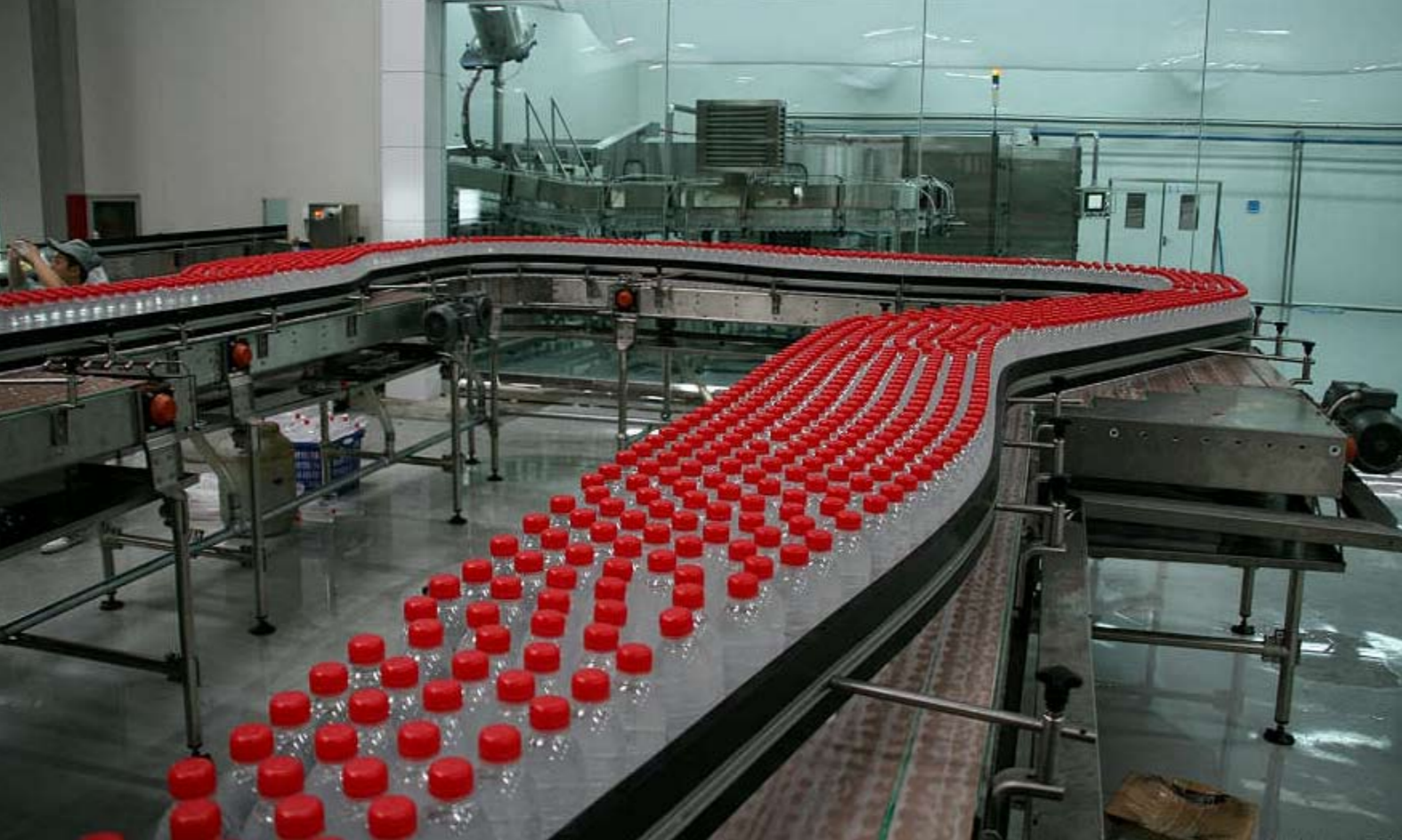
达意隆36000BPH灌装线在杭州农夫山泉运转 Tech-Long 36,000 BPH filling line running smoothly in the producing site of Nongfu Spring, Hangzhou
