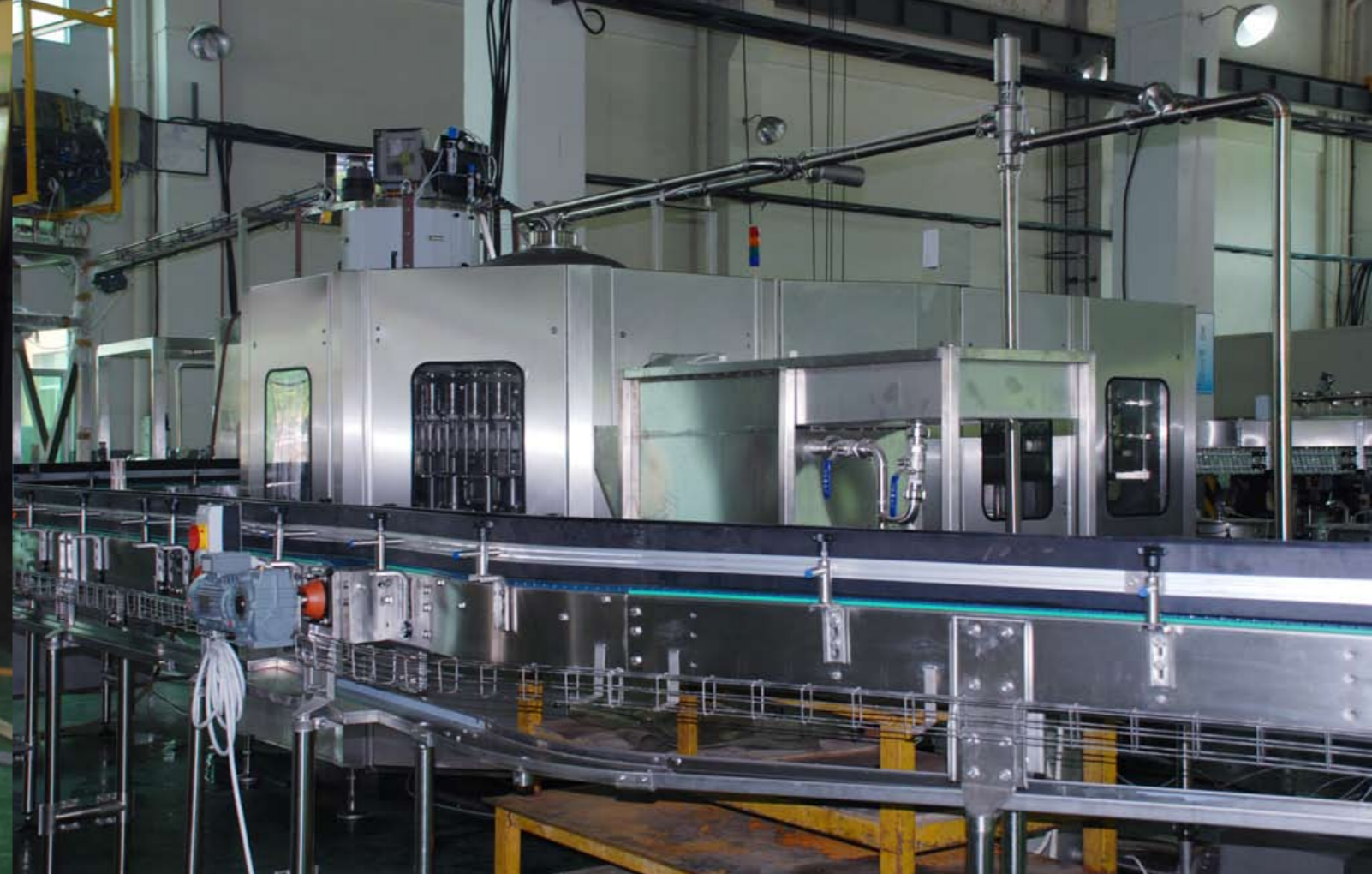
达意隆24000BPH热灌装线调试现场 Commissioning of 24,000 BPH hot bottling line
