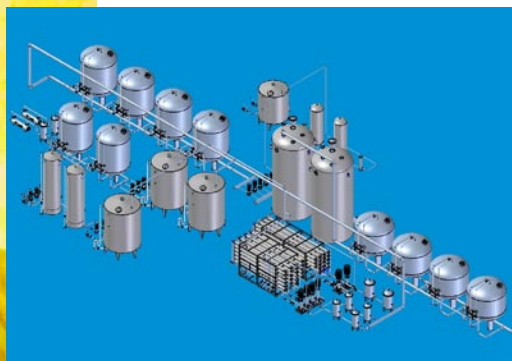
顺德龙江生力项目达意隆水处理系统管道布局图 Pipeline arrangement of Tech-Long water process system of San Miguel project, Longjiang, Shunde
