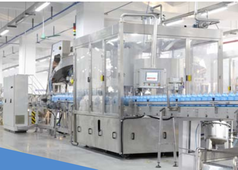
灌装、旋盖（压盖）二合一一体机 Two-in-one filling and capping (crowning) equipments
