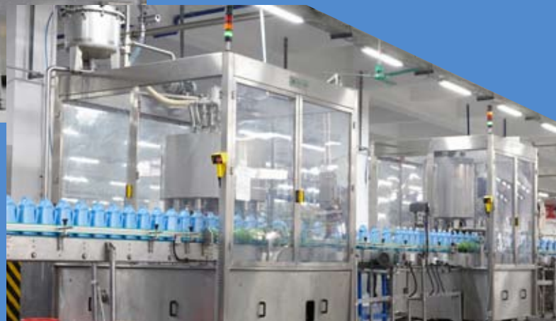
灌装、旋盖（压盖）分体机 Split type filling and capping (crowning) equipments
