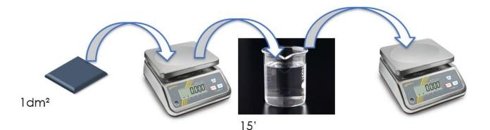
Dye spot test (one test per coil performed)
