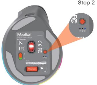
Short press the mode switch button at the bottom of the mouse, the \$1 blue light flashes slowly
