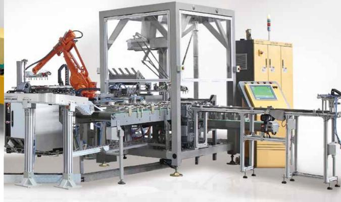
Robot labeller, a self-developed product of our company, mainly consists of parallel robots, label stripping mechanism, positioning mechanism and conveying line, and it is an advanced labeling device in China.
