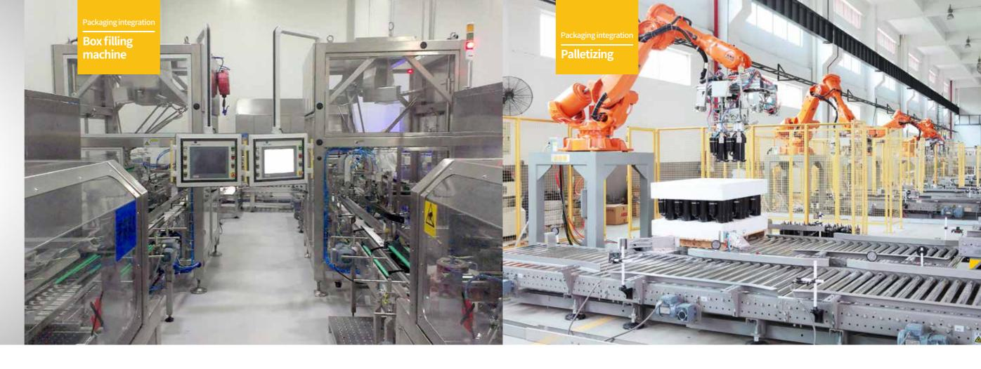
Visual precise positioning is adopted for the robot sorting line; the robot can grab fast and accurately with the vacuum chuck or pneumatic clamping jaw.
