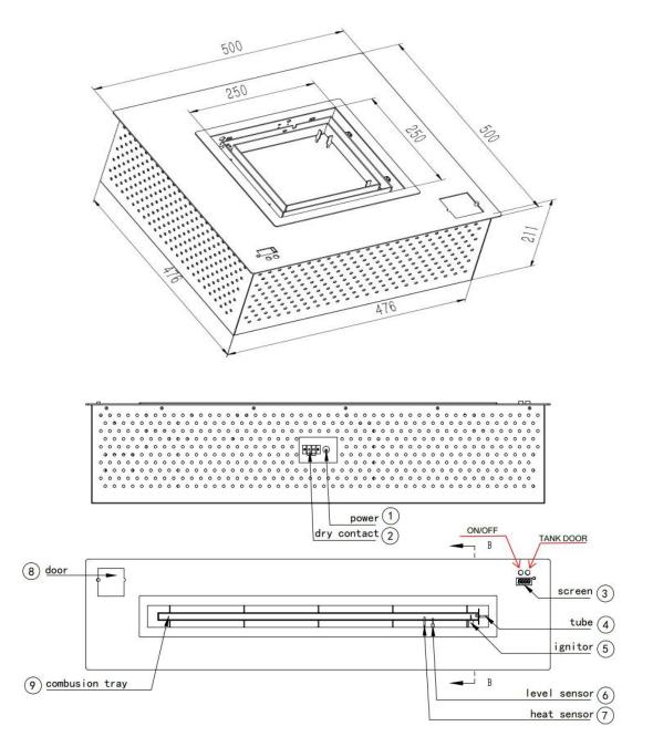
1, Before connecting electronic power to the burner, close the tank door well.
